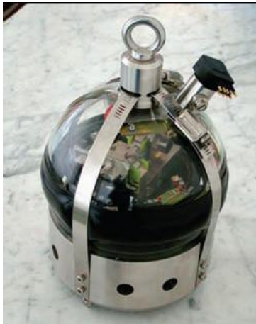
Figure 9 CGM-40TOBS Guralp self-levelling base
