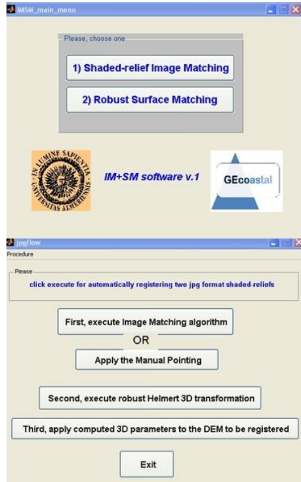
Fig. 3 Software developed to carry out the proposed methodology based on Matlab® code.
