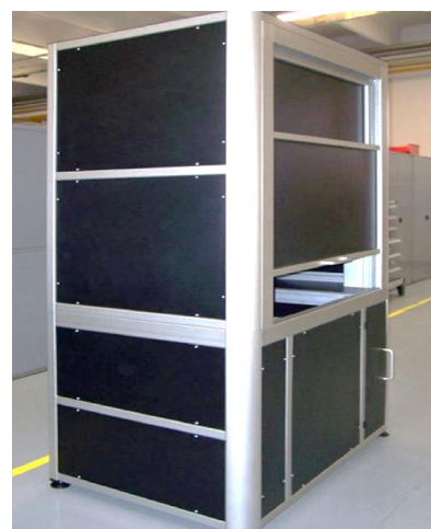
Fig. 9 Dyeing machine external cabin.
