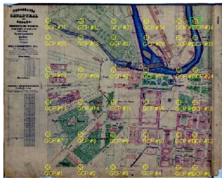
Fig. 3 Example of the points of support distribution on the HK 31L image.
